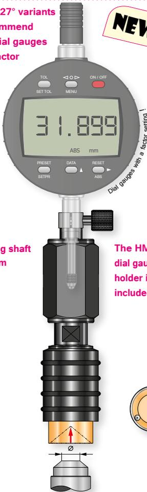
Clamping shaft Ø 8h7mm
